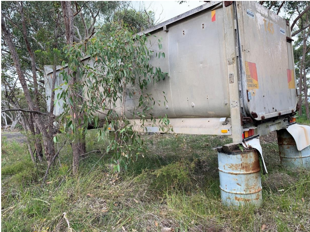
PHOTOGRAPH 7 Truck trailer elevated using drums
